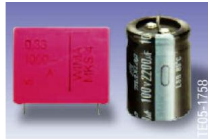
Left: Non-polarized capacitor Right: Polarized capacitors
